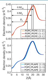
**Figure 8.** Total electron density profiles for different POPC/POPE (upper panel) and POPC/PLAPE (lower panel) mixtures obtained from MD simulations at 310 K with POPC/POPE and POPC/PLAPE molar ratios listed in the legend. Rough locations for the thickness metrics are shown in the top panel (exact values are provided in Table 2).
