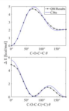
Figure 5. Potential energy scan about dihedrals of 1-ethoxypropene: (top) C-O-C=C and (bottom) C-O-C-C(=C); QM using MP2/cc-pVDZ//Eint[MP2:CC] (black) plotted with results after dihedral fitting (blue). Other torsions remained trans.
