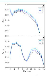
**Figure 10.**  $S_{\rm CD}$  calculations of POPC sn-1 (A) and sn-2 (B) chains from MD simulations of POPC/PLAPE mixtures at 303 K with POPC/PLAPE molar ratios listed in the legend. Here carbon-based order parameters are given. For the sn-2 chain, the two hydrogens attached to carbon-2 have a different splitting; therefore, the  $S_{\rm CD}$ s of 2R and 2S are shown separately instead of their average.
