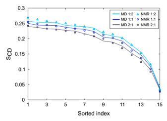
**Figure 9.** Comparison of POPC sn-1 chain  $S_{\rm CD}$  obtained from simulations with experimental  $^2{\rm H}$  NMR measurements at 303 K using a decreasing monotonic sorting of order per methylene segment. The latter takes into consideration that  $^2{\rm H}$  NMR order parameters lack assignment for a specific carbon atom along the chain. The POPC/PLAPE molar ratios are listed in the legend.
