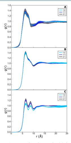
**Figure 11.** Comparison of two-dimensional radial distribution functions (RDFs) of PLAPE-PLAPE (A), PLAPE-POPC (B), and POPC-POPC (C) in POPC/PLAPE mixtures. The results are from simulations carried out at 310 K with POPC/PLAPE molar ratios listed in the legend.
