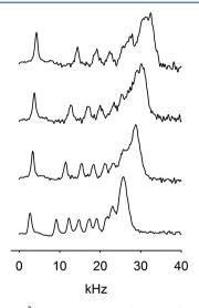
**Figure 3.** DePaked  $^2$ H NMR spectra of POPC- $d_{31}$  and POPC- $d_{31}$ / PLAPE mixtures at molar ratios of 2:1, 1:1, and 1:2 (from bottom to top) recorded at 30.0  $^{\circ}$ C. Spectra were recorded within 1 h of sample preparation when oxidation of the plasmalogen double bond of PLAPE was negligible.
