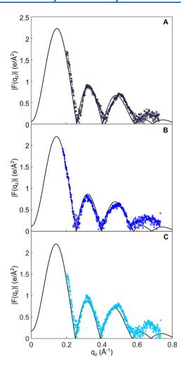
**Figure 7.** X-ray form factors  $(|F(q_z)|)$  as a function of the scattering angle  $(q_z)$  obtained from simulations at 310 K (black line) of three POPC/PLAPE molar ratios: (A) 2:1, (B) 1:1, and (C) 1:2. The simulation results (solid line) are compared to experimental results (dots). Calculated goodness of fit between form factors obtained from simulations and from experiment of POPC/PLAPE molar ratios is 0.019 for 2:1, 0.016 for 1:1, and 0.022 for 1:2.
