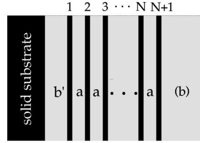
FIG. 4. Schematic of a stack of  $N+1$  bilayers on a solid substrate. Mean spacing between bilayers is  $a$  and the space between the stack and the substrate is  $b'$ . The water (gray area) extends far to the right of the stack when the stack is immersed in liquid water and extends a distance  $b$  when the stack is in vapor.
