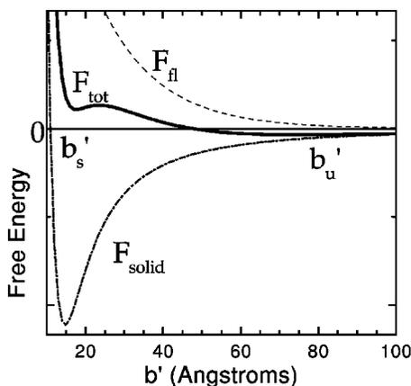
FIG. 5. Fluctuation free energy  $F_{fl}$  and interaction with solid substrate  $F_{solid}$  versus  $b'$  with the sum  $F_{tot}$  indicated by a solid line. This loosely unbound stack has  $b' = b'_u$ , which undergoes a transition to  $b'_s$  with application of osmotic pressure. Free energy scale is unknown.
